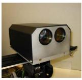
Laser source: 1.54 um - erbium fiber laser Transmitter: 0.8 W Output power Aperture diameter: Receiver: Aperture diameter 50 mm Field of View 75 µrad InGaAs photodiode 100 x 100 µm<sup>2</sup> 60 MHz Intermediate frequency: one AOM (40 MHz) in the transmitter beam one AOM (100 MHz) in the LO beam
